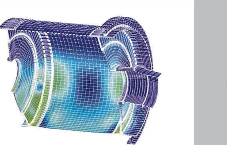
The OPSIM Ball Mill Body is a critical component in the grinding process of various materials. It is designed as a low-speed rotary cylinder mounted on two large bearings horizontally. Inside the cylinder, grinding media such as steel balls are placed. These balls are lifted to a certain height by the action of centrifugal force and friction, and then they fall or drop to grind the material inside the mill.
